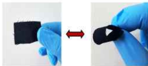
Fig. 9. Photograph of PANI grafted on the plasma-pretreated flexible polyester fabric.
